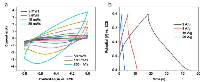
Fig. 4. The NMN@PPy anode electrochemical performance. (a) The CV NMN@PPy anode CV curves; (b) The NMN@PPy anode GCD curves.
