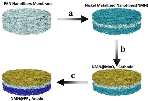
Schematic 1. The illustration of fabrication process of all-in-one ultrathin flexible asymmetric supercapacitors: (a) Sputtering and electrodeposition nickel onto the two sides of electrospinning nanofibers membrane, and the middle part without metallized as separator. (b) Electrodepositing a layer  $\text{MnO}_2$  onto upper side of metallized nanofibers as the cathode. (c) Electrodepositing a layer PPy onto lower side of metallized nanofibers as the anode.
