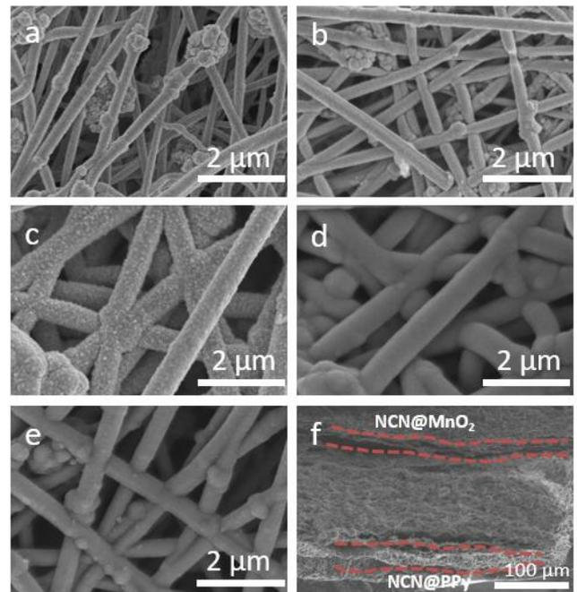
Fig. 1 (a) The SEM of PAN nanofibers; (b) The SEM of nanofibers after magnetron sputtering nickel; (c) The SEM of nanofibers after electrodeposition nickel; (d) The SEM of  $\text{NMN@MnO}_2$ ; (e) The SEM of  $\text{NMN@PPy}$ ; (f) The cross-sectional SEM of all-in-one ultrathin flexible asymmetric supercapacitors.
