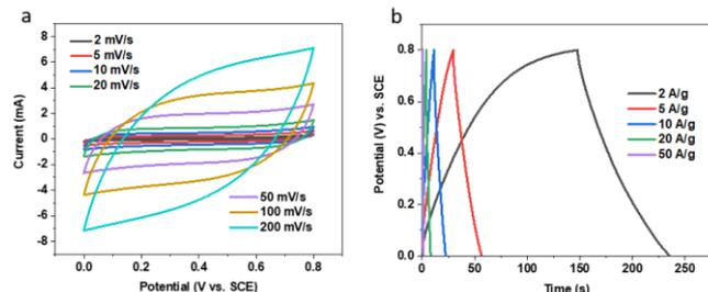
Fig. 3. The NMN@MnO<sub>2</sub> cathode electrochemical performance. (a) The NMN@MnO<sub>2</sub> cathode CV curves; (b) The NMN@MnO<sub>2</sub> cathode GCD curves.
