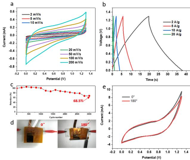
Fig. 5. The all-in-one ultrathin flexible supercapacitors electrochemical performance. (a) The coin type cell CV curves; (b) The coin type cell GCD curves; (c) The coin type cycling stability; (d) The photograph of a pouch type cell (size:6 cm $\times$ 5 cm); (e) The pouch type cell CV curve at the scan rate of 50 mV/s in different bending angles.
