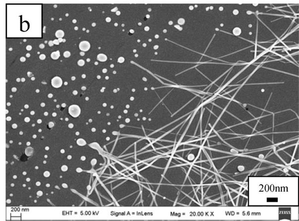
Fig. 5 (a) SEM image of the AgNWs/EVA composite film after the laser patterning process. (b) Magnified side-view SEM image of the edge of the conductive road, showing that the AgNWs were melted into small silver balls. We could clearly see the laser path where the AgNWs were melted into small silver balls to cause the open circuit and form a conductive road.
