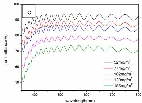
Fig. 1 (a) SEM image of the AgNWs/EVA composite film on a PET substrate; (b) Magnified SEM image of the AgNWs/EVA composite film, showing the diameter of the Ag NWs (diameter ~25nm); (c) The optical transmittance spectra of the transparent film samples with different AgNWs concentrations. With the increase of AgNWs concentration, there was a decrease of the transmittance. The unusual wavy curves are related to the PET films that we used, which is an interesting phenomenon yet to be explored .
