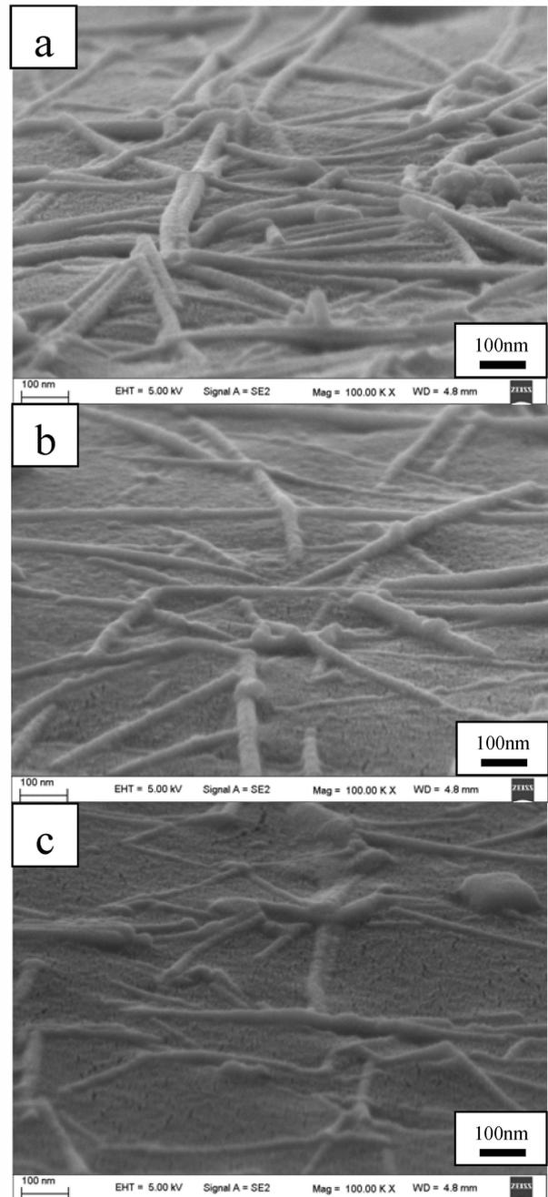
Fig. 3 With different heating time, the AgNWs on the EVA shows different morphologies; AgNWs was gradually embedded in the resin as the time went on for (a) 1 min; (b) 5 min; (c) 10 min.
