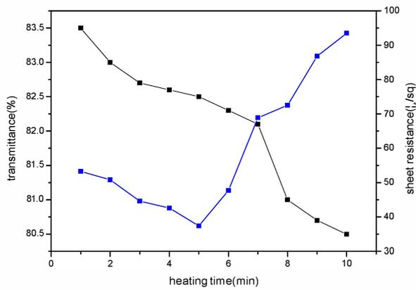
Fig. 2 Variation of transmittance and conductivity over different heating time.
