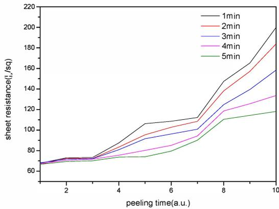
Fig. 4 The peeling test of AgNW/EVA/PET films with different heating times.
