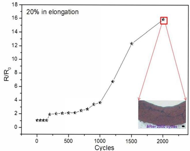
Fig. 6 Normalized resistance of Cu circuits vs. stretching cycles with a constant elongation of 20%. The insert is optical image for Cu circuits after 2000 stretching cycles (the scale bar is 50  $\mu$ m).
