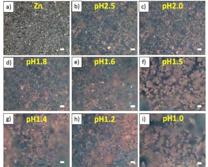
Fig. 2 Optical microscopic images of original Zn paste (a) and r-Cu reduced from  $\text{Cu}^{2+}$  containing solution with a pH value of 2.5 (b), 2.0 (c), 1.8 (d), 1.6 (e), 1.5 (f), 1.4 (g), 1.2 (h), and 1.0 (i). All scale bars are 5  $\mu\text{m}$ .
