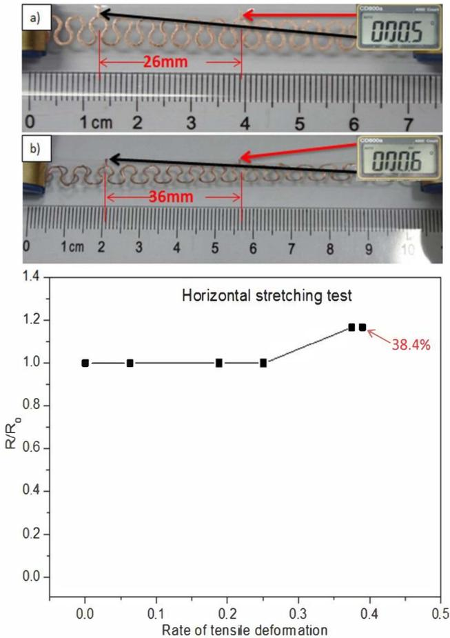
Fig. 5 Optical microscopic images of longitudinal stretching test for e-Cu circuits before (a) and after (b) stretching (Top) and Normalized resistance of e-Cu circuits vs. rate of tensile deformation (Down). (Note: the red and black arrows represent the probes of digital multimeter in a) and b))
