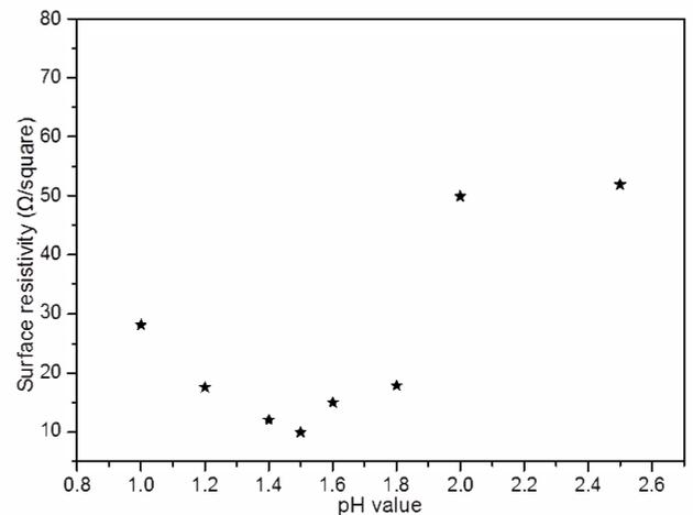
Fig. 3 The surface resistivity of r-Cu layer versus pH value of  $\text{Cu}^{2+}$  containing solution ( $30 \pm 2 \mu\text{m}$  in thickness for all conductive circuit layers).
