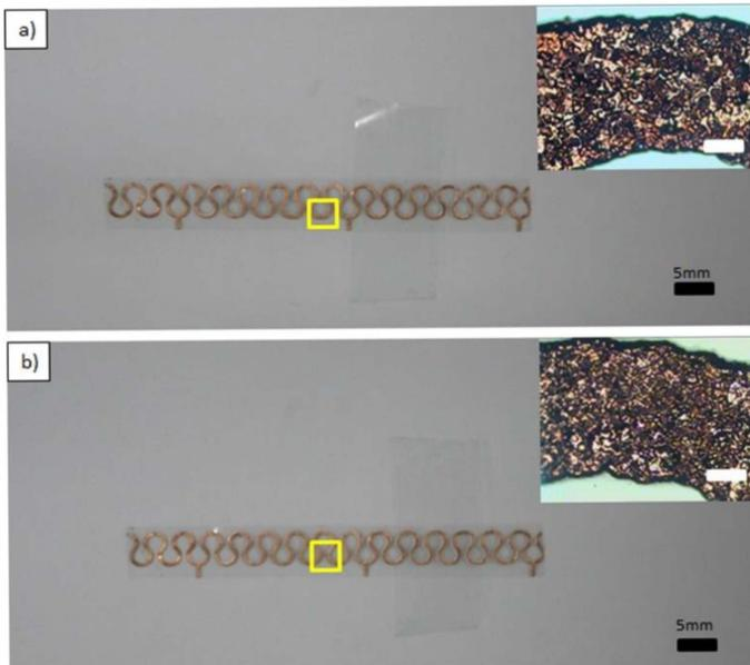
Fig. 4 Photographic images of the Cu circuits a) before and b) after tape peeling. The inserts are optical microscope images of the selected area. The scale bars of a) and b) are 5 mm. The scale bars of the inserts are 50  $\mu$ m.
