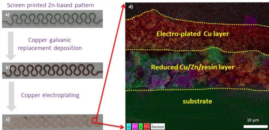
Fig. 1 a) photographic image of printed Zn pattern; b) photographic image of the sample after galvanic replacement deposition of Cu; c) photographic image of the sample after electroplating; d) SEM-EDS mapping image of the cross section views of the conductive circuit after copper electroplating.
