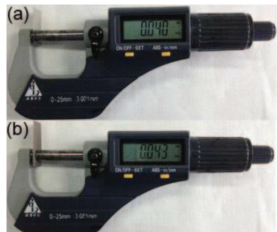
Fig. 3 the thickness of current collector before and after electro-deposition
