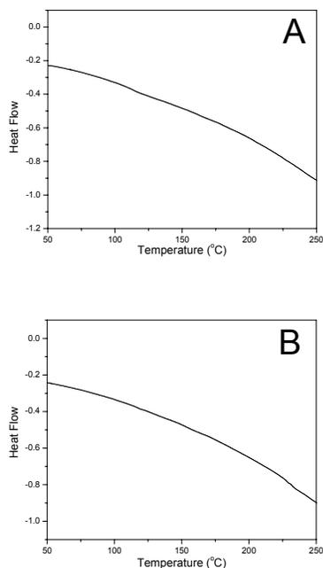
**Figure 7. DSC heat flow curves of the silver flake samples. (A) Control sample (without silver surface pretreatment); (B) 0.2% chemical A pretreatment.**
