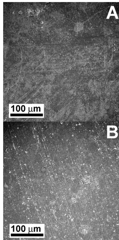
Figure 5. SEM images of the lap shear fracture surface (without aging). (A) control sample, (B) ICA samples with 0.2% chemical A treated silver flakes (magnification: 250x).
