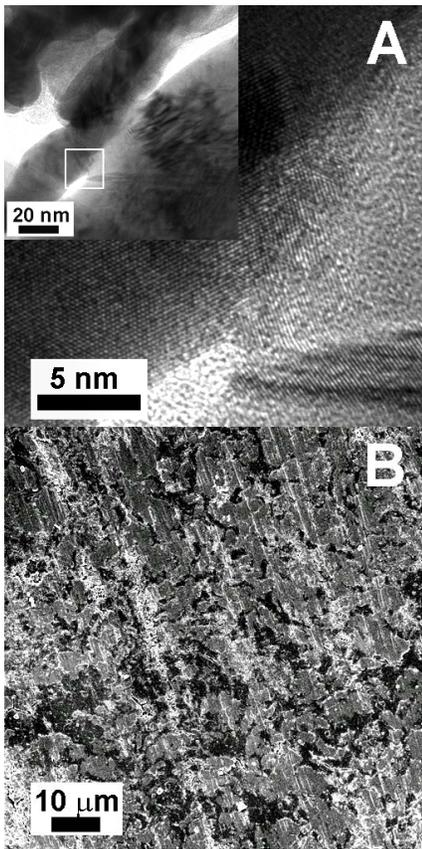
Figure 3. (A) A HRTEM image of the chemical A modified (0.2%) silver flakes in the ICA samples. The white square in the inset image shows the magnified part of the image. (B) SEM image of the cross section profile of the same sample.
