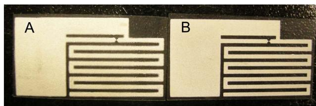
**Figure 2. Photographic images of the screen-printed ICA samples. (A) 0.2 wt% chemical A modified silver in its ICA formulation (75 wt% silver); (B) control sample (bare silver) in its ICA formulation (75 wt% silver).**
