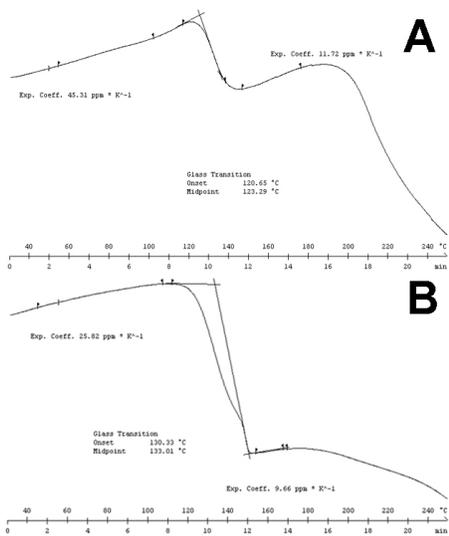
**Figure 6. Thermal expansion curves from the CTE analysis of fully-cured ICA samples (A) control sample (without surface modification of silver); (B) ICA sample with 0.2% chemical A surface treatment of silver.**
