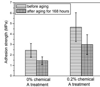
Figure 4. Adhesion strength test in the 85°C/85%RH aging test of the ICA samples with 0.2% chemical A treated silver flakes.
