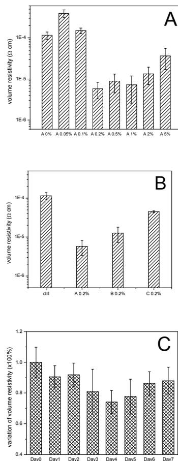
**Figure 1. Volume resistivity of the ICAs in different conditions. (A) volume resistivity of the ICAs with 75 wt% silver filler loadings. (x-axis shows the chemical A content to silver flakes.) (B) Volume resistivity of the ICAs with 75 wt% silver filler loadings (x-axis shows the chemical A, B, C and control sample). (C) Volume resistivity change of the ICA with 75 wt% silver filler loading (chemical A content is 0.2 wt% to silver) in an  $85^{\circ}\text{C}/85\%\text{RH}$  aging test.**
