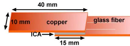
Scheme 1. A schematic illustration of a lap shear test specimen. The ICA is filled in between and the thickness of the ICA is 200  $\mu\text{m}$  (controlled by the glass fibers).
